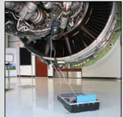
DTT motor installed on a gear box
