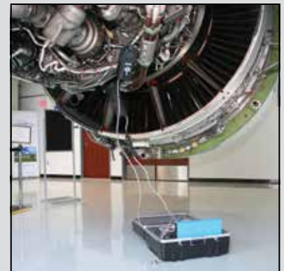
DTT motor installed on a gear box
