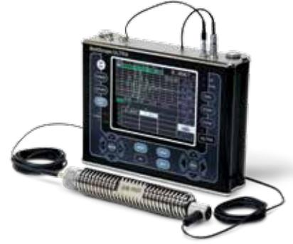
The Ultra is a powerful unit which can monitor almost any length of fastener while maintaining constant signal and strength. The Ultra is designed to verify any application that requires close load tolerances on fasteners. Loaded and un-loaded bolt readings can be displayed on a large colour easy to read screen at any time throughout the bolts' active service life. The device can be configured for linear regression or vector readings to assist load measurement optimisation.
