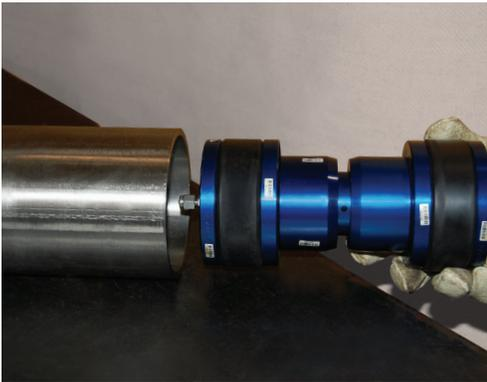
**Above** Dual-purpose inline isolation and weld test tool is inserted into a cut pipe
