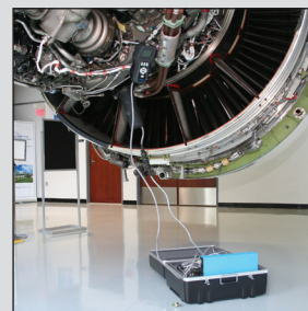
DTT installed on a gear box
